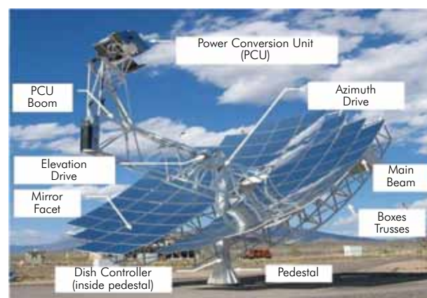
Figure A.10: Dish-Engine Photo with Major Component Identification
