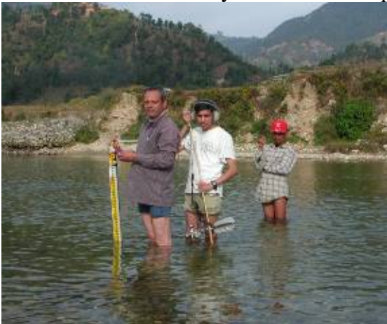
Figure 2.17: Discharge measurement at the Andhi Khola upstream of the Badh Khola confluence on 9 December 2007.
