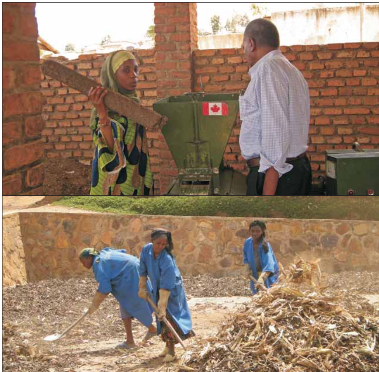
COCEN manager demonstrates the compressing of waste into fuel briquettes (top)
