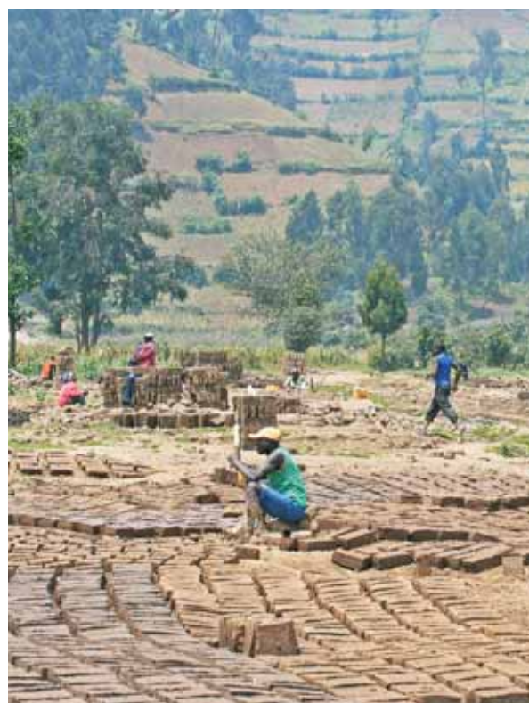
Residents in Nyabihu District produced sun-dried adobe bricks to reconstruct their homes destroyed by flood
