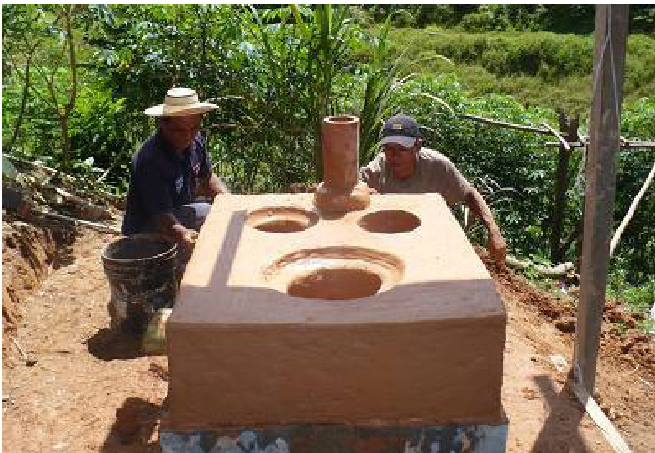
Ecological wood stoves, spend less wood than a traditional stove. (Source: elsiglo.com )
