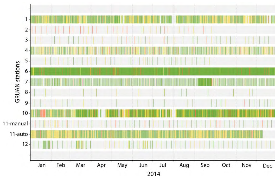
Figure 85. Quality assessment of data from Vaisala RS92 radiosonde ascents made by 12 GRUAN stations in 2014. Results for one station are shown separately for manual and automatic launches. Coloured vertical lines represent ascents, with colour indicating the quality flag. Green denotes data that have been processed, passed all quality checks and archived at NCEI as GRUAN measurements. Yellow denotes data that have been processed but failed one or more of the strict GRUAN quality checks. Red denotes ascents that could not be processed or for which it is known that operational procedures were not followed completely.
