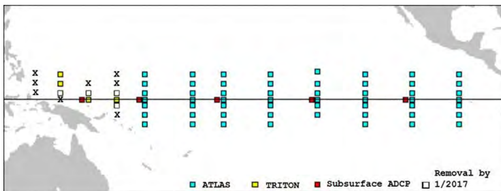
Figure 47. Status of the TAO/TRITON mooring array. “x” marks where TRITON moorings have already been removed
